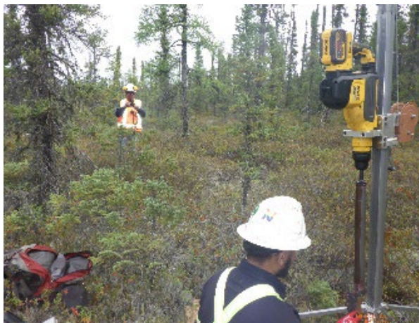
Figure 4. Talon drill used for sampling peat
